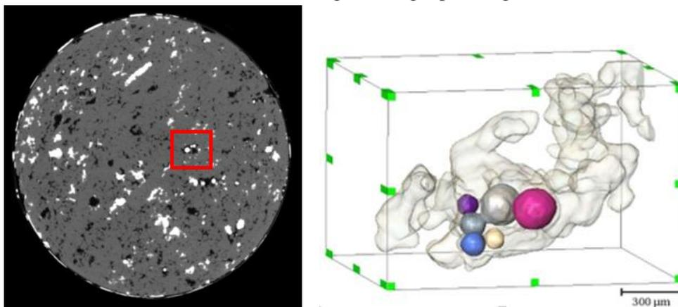
Figure 2 - Example of a carbonate rock (left) saturated with a NAPL phase (bright) and water (dark phase) and (right) the 3D rendering of the segmented pore space with the fluid inclusion.
