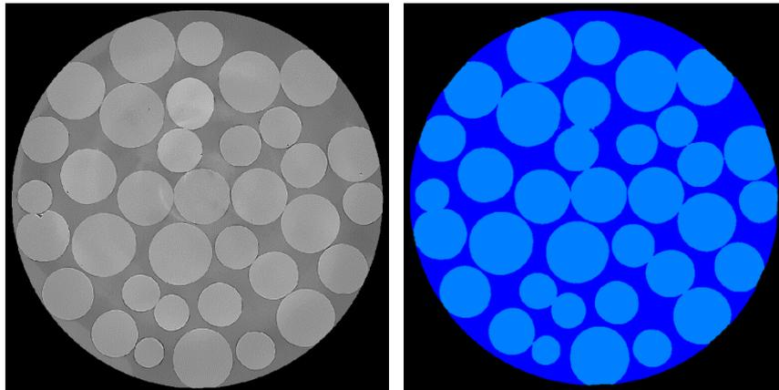
Figure 1 – (Left) Raw image of glass beads (left) and the correspondent segmented image (right). The sample diameter is approximately 4 mm and the pixel size is 3.2 $\mu$ m.
