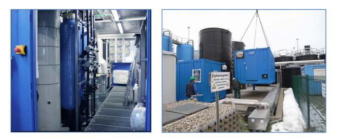
Fig. 1: View into one of two *Treatment Train* containers and placement of the units at a field site for plot testing.
