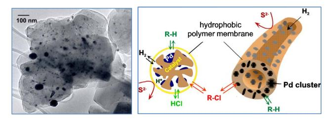
**Fig. 2:** A hydrophobic zeolite Y wet impregnated with Pd (left) and Pd embedded in a hydrophobic polymer membrane (right) to protect catalysts from sulfur poisoning in the water phase.
