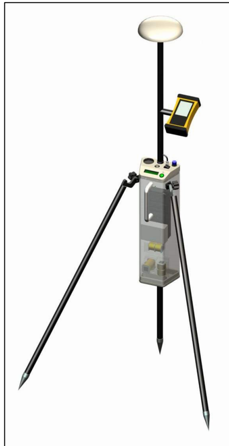
Figure 1 - The Willowstick instrument, which captures magnetic field strength data.
