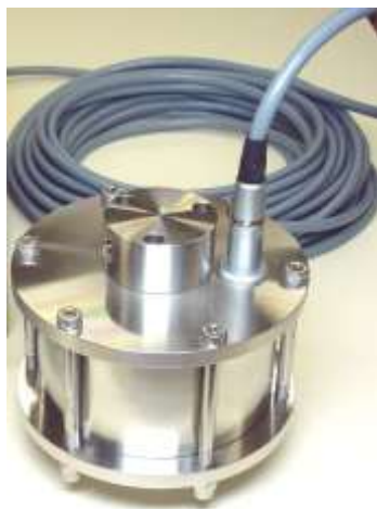
Figure 4. GGUN-FL30 Field fluorometer probe. 160mm diameter.
