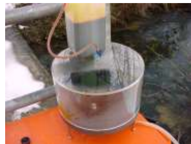
Figure 2. Enclosure protection against the wind. A Mariotte bottle delivers the tracer solution at a constant rate.
