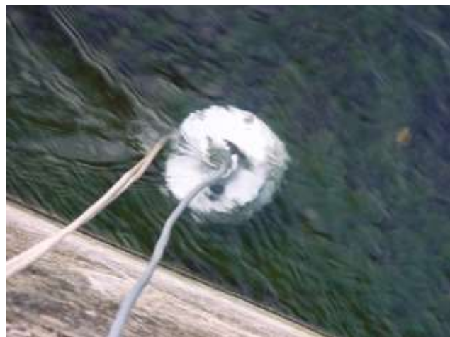
Figure 5. Immersion in water. Mass of the probe: 7.5 kg
