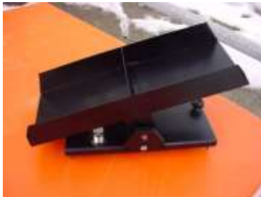
Figure 1. Tipping bucket. The capacity of a bucket is 110 ml.
