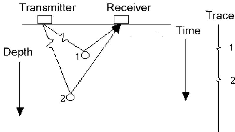
**Figure 2.** Basic principle of the GPR method. The transmitter antenna emits a pulse that reflects on the two targets (1 and 2) before being recorded by the receiving antenna. The time information in the trace (reflections 1 and 2) can be converted to depth as long as the velocity of electromagnetic waves is known. The antennae can be moved along a profile in fixed offset or in CMP field configurations.
