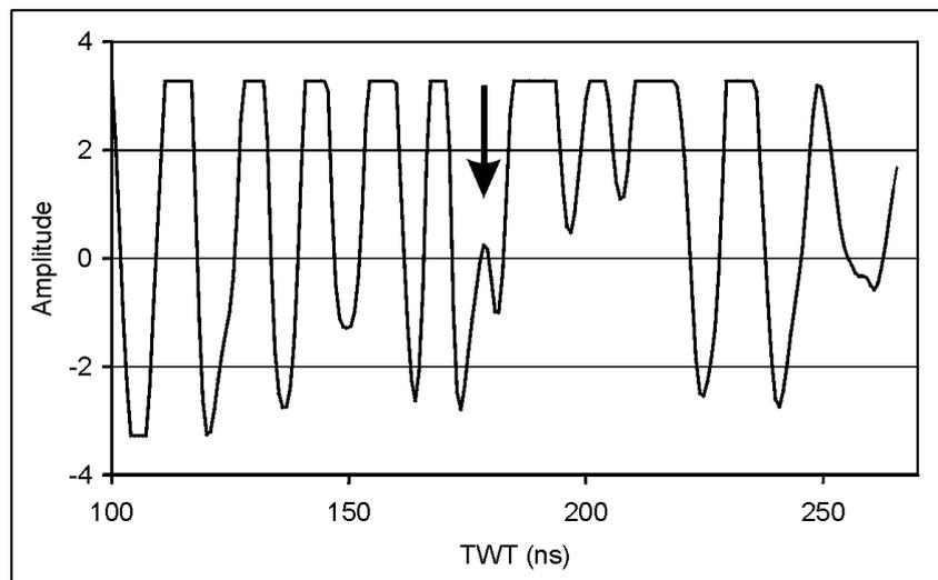
**Figure 5.** End section of trace at 35 m. The arrow shows the first of a series of phase inversions, occurring at the top section of the water-filled fractured rock. Amplitudes are clipped at a maximum of 3.2. The vertical scale is arbitrary.
