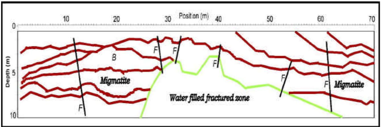
**Figure 6.** Interpretation of the radar section shown in Figure 4. *F* are interpreted fractures and *B* is interpreted as a boudin structure.
