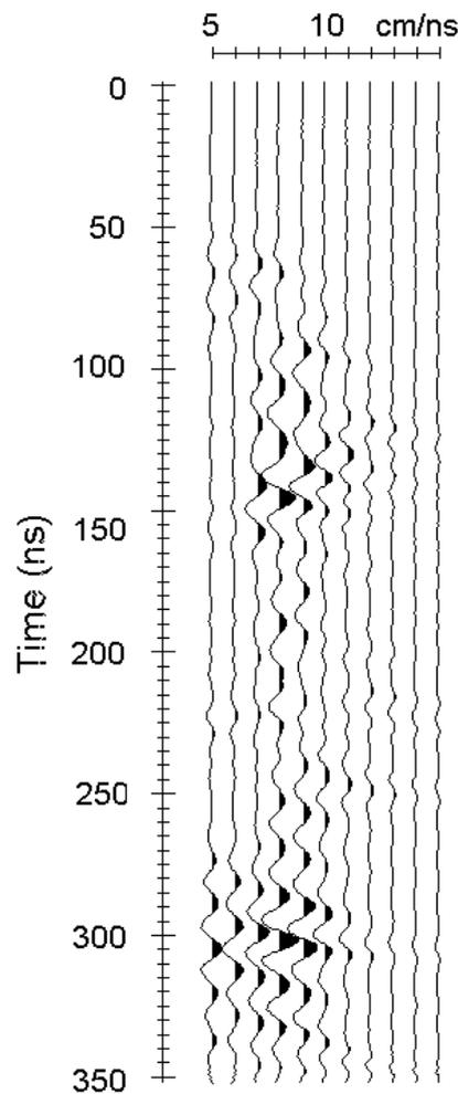
**Figure 3.** Velocity analysis for the CMP profile. Velocity is incremented in 1 cm/ns steps from 5 to 15 cm/ns.
